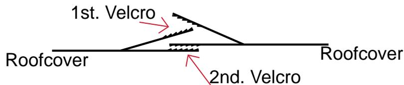
Use the velcro overlay to attach 2 roof sections to each other.
