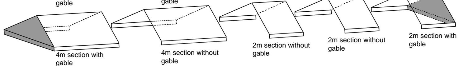
When you are making your CombiTent **shorter**. Use the velcro overlay to detach roof sections.
